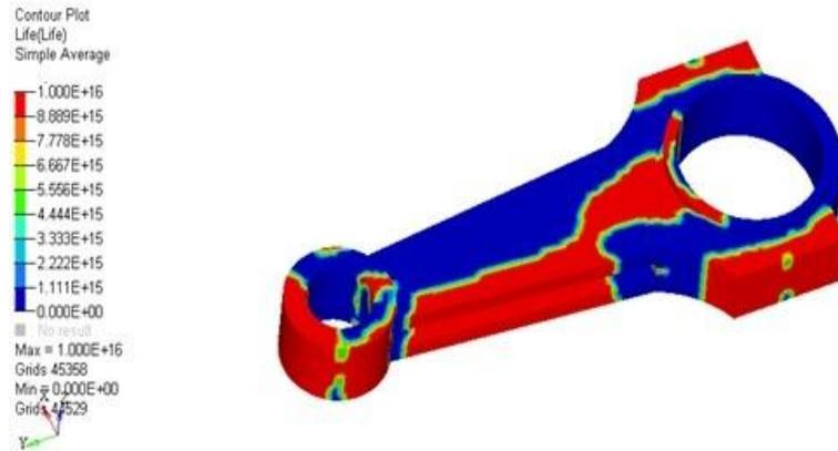
Figure 4: Life of the powder metal component is 1E16 cycles
