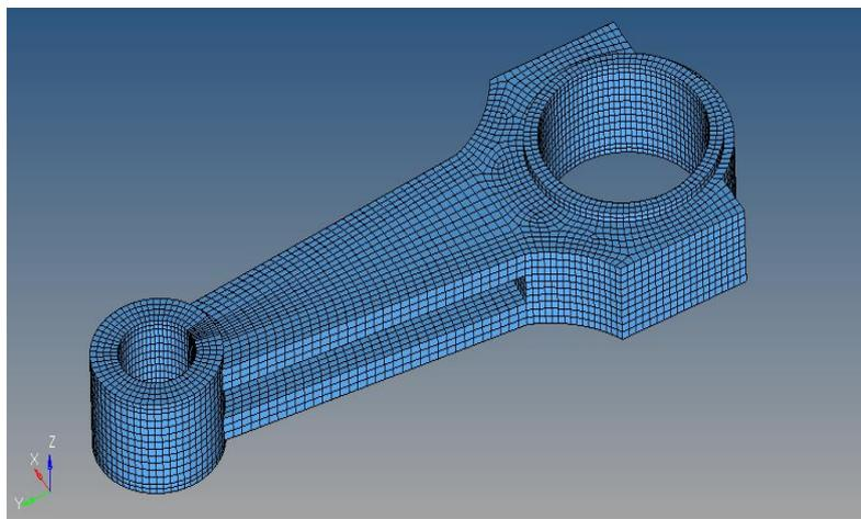
**Figure 1:** Hexamesh using Hypermesh
