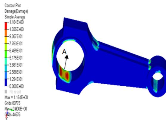
**Figure 3:** forged steel rod damage (A)
