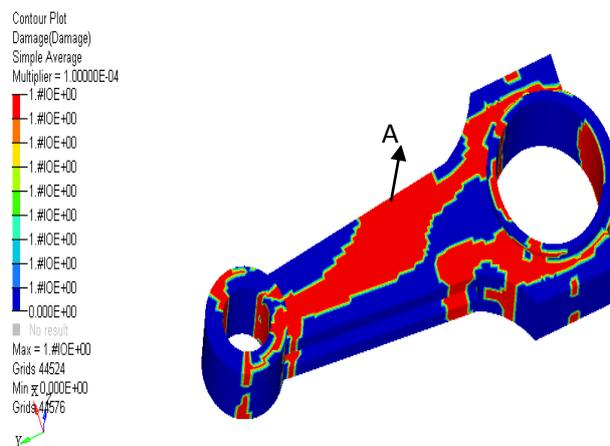
Figure 5: Powder metal connecting rod get damages (A)
