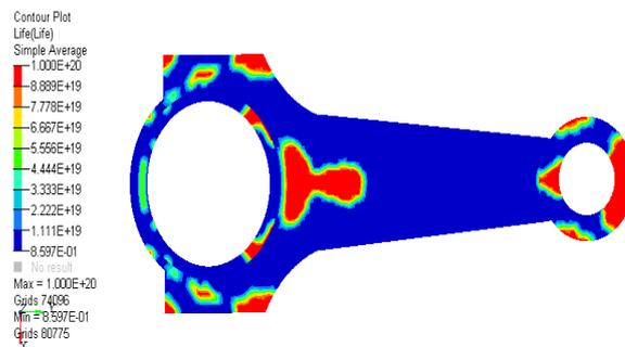
**Figure 2:** Life of the forged steel component is 1E20 cycles
